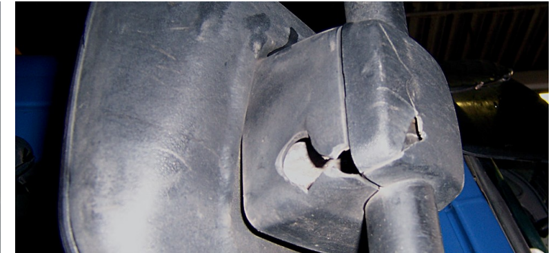
✘ Mirrors/impact damage • Deep scratches, crack formation or material chipping
