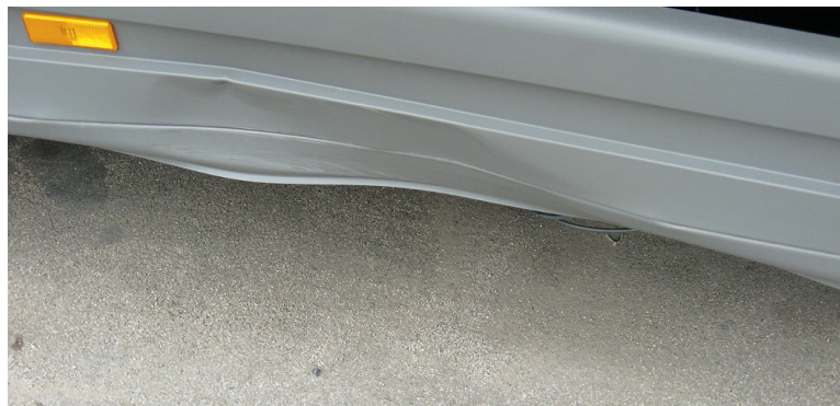
✘ Side impact protection/impact damage • Major deformations
