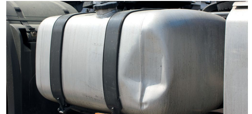
✘ Tank/impact damage • Deformations
