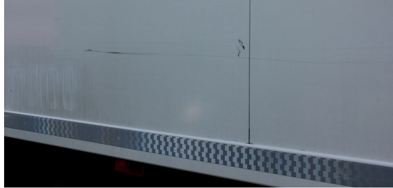
✔ Box body/signs of use • Scratches caused by scraping
