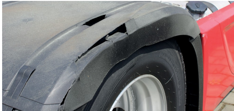
✘ Wheel cover/impact damage • Holes or deformations
