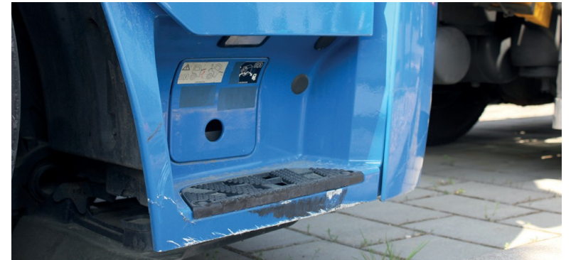
✘ Entrance/impact damage • Deep scratches, material ablation or crack formation
