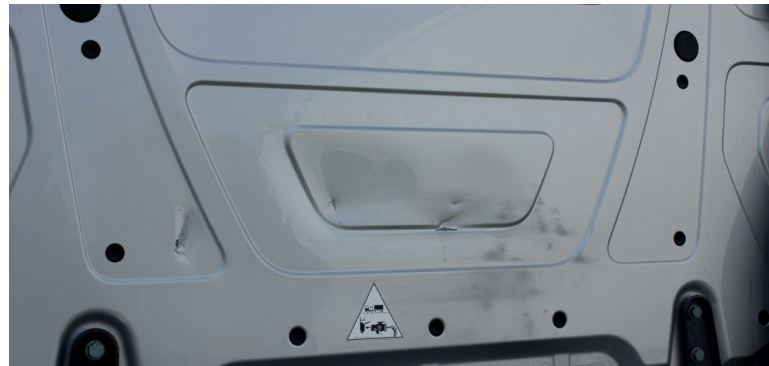
✘ Rear of cab/impact damage • Dents, damage to paintwork, dented or cracked
