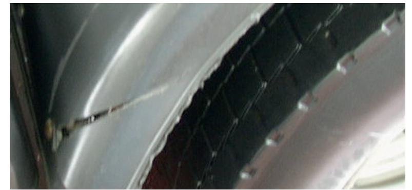
✘ Wings/impact damage • Scratches, crack formation or material chipping
