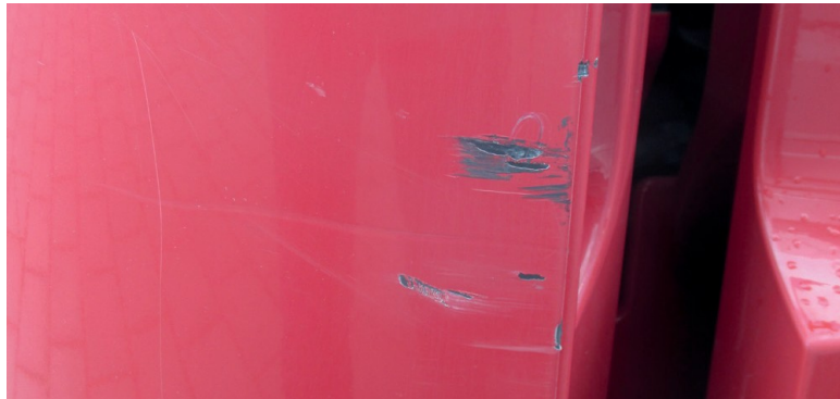
✘ Wind deflector/impact damage • Scratches, cracks or fractures
