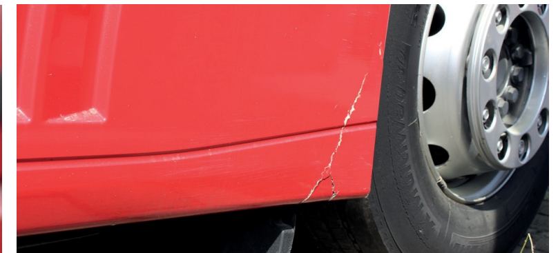
✘ Side protection cladding/impact damage • Scratches, cracks or fractures
