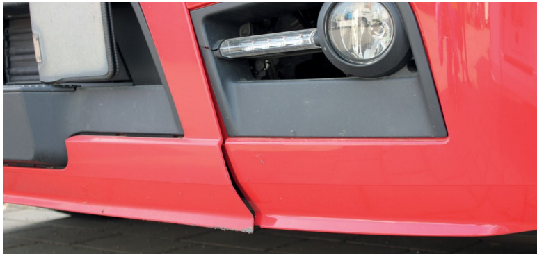
✘ Bumpers/impact damage • Major scrapes, crack formation or material fractures
