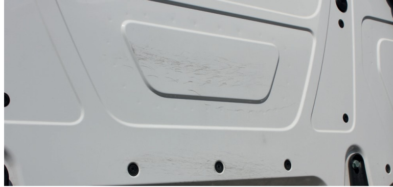
✔ Rear of cab/signs of use • Minor scratches, small dents or chafe marks
